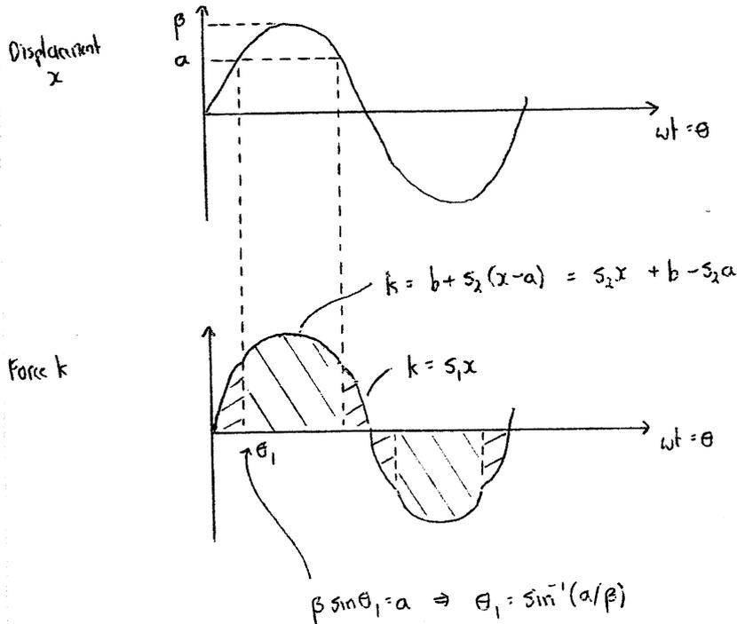
$$D = \frac{1}{\beta\pi} \int_0^{2\pi} (\text{output}) \sin \theta \, d\theta = \frac{1}{\beta\pi} \left\{ k \int_0^{\theta_1} (s_1\beta \sin \theta) \sin \theta \, d\theta + 2 \int_{\theta_1}^{\pi-\theta_1} (s_2\beta \sin \theta + b - s_2a) \sin \theta \, d\theta \right\}$$
