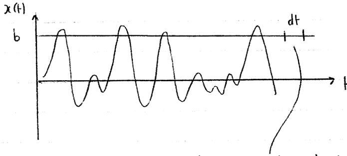
to cross in a time interval  $dt$  with velocity  $> u$ , must have
