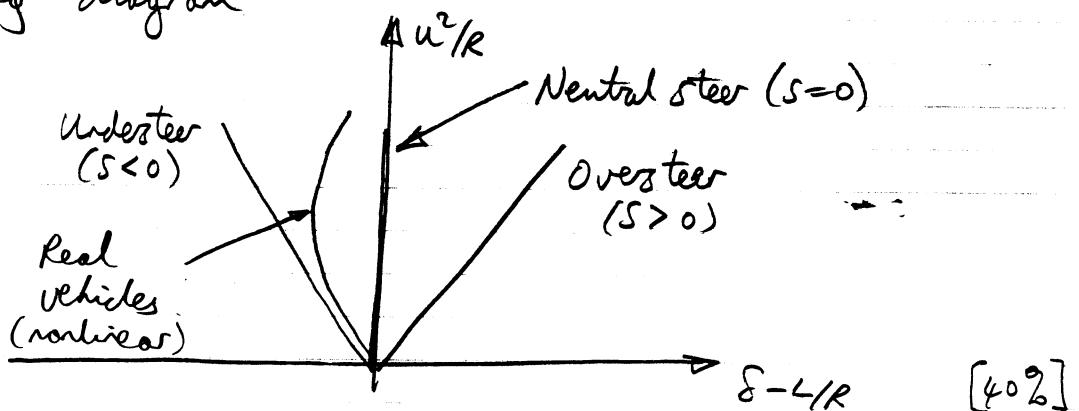
(c) Real vehicles understeer at low speeds & oversteer at high speeds. This is caused by two main effects
