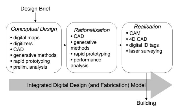
In the above diagram, flow of information generally moves from left to right often with many iterative loops within one stage. For example, geometric data from digitising a 3D model can be used as the basis for a CAD model that is further developed. Generative methods can then be used, e.g. for generating cladding or stone patterns, and the new design in the form of a CAD model is then used as input to rapid prototyping and/or analysis tools both of which feedback on the original CAD model.
