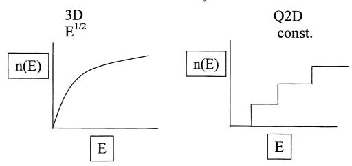
Electrons in a 2-DEG are confined in one direction (z), and free to move in the other two (x, y). To be general,
