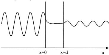
If we say that the amplitude of the incident wave is 1, then the wave-function in the barrier region is:
