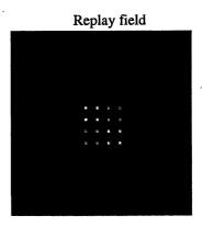
The hologram is an array of pixels in either phase or intensity which will generate a desired replay field. The relationship between the two is via the Fourier transform which converts one into the other and is reversible. The FT can be done by either a positive focal length lens or by going into the Fraunhopher region of free-space.
