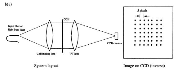
ii) The square shape of the pixels in the CGH means that there will be an overall sinc (sine(x)/x) shaped envelope in the replay field.
