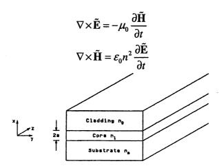
In a slab waveguide such as that shown above, the electromagnetic fields E and H do not have a y dependency due to the geometry of the waveguide. Hence we set  $\partial \mathbf{E}/\partial y = 0$  and  $\partial \mathbf{H}/\partial y = 0$ . Putting these relationships into the ones above gives us two independent electromagnetic modes denoted as the transverse electric TE and transverse magnetic TM modes.
