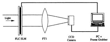
The input and reference images are displayed side by side on a FLC SLM as in a full JTC. The SLM is illuminated by a collimated laser beam and the images are Fourier transformed by a single lens in its focal plane. This spectrum is then imaged onto a CCD camera. The spectrum is then non-linearly processed before being displayed onto the SLM again to form the correlation information. The 1/f JTC is a two-pass system, using the same lens to perform the second Fourier transform.
