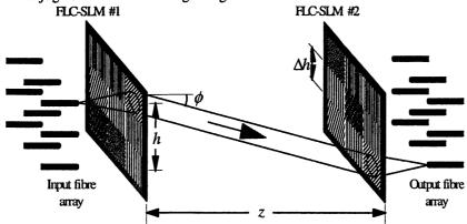
The two hologram switch can be scaled to any size and the loss through the switch does not scale with the number of input and output ports, it does however increase the loss as there are now two holograms routing the same beam. The only parameters which scale with the number of ports are the crosstalk and the physical length z. The crosstalk of the two hologram switch is greatly improved as the crosstalk of the first hologram is multiplied by the cross talk of the second hologram.
