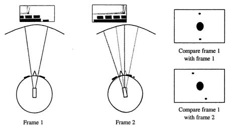
The position of the correlation peaks tells us how much one frame has moved from the previous one when the pilot's head rotates, hence by measuring the distance and knowing the dimension between the pilot and the cockpit, we can sense how much the head has rotated and therefore track it.
