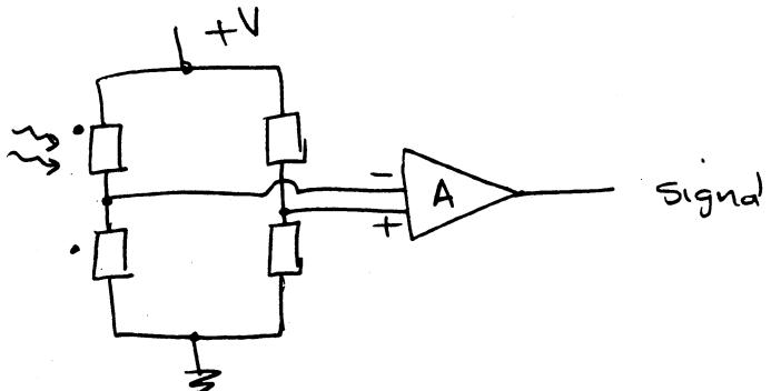
A pair of sensors compensates for ambient temperature changes - it would be practically impossible with a single resistor to detect small temperature changes. Also, the compensated pair cancels the effect of self heating due to the bridge excitation.
