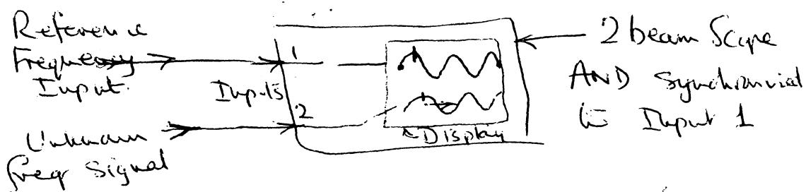
The Time T, measured by stopwatch, for the lower frequency trace display to drift to the ~~right~~ left (fewer cycles in given time) (or vice-versa for higher frequency), by a no of whole cycles, say ~~say~~ 10.
