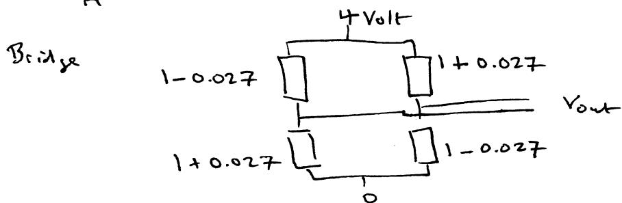
$$V_{\text{output}} = 4 \times 0.027 = \underline{0.11 \text{ Volt}}$$
