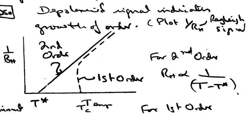
Couple with Scanning Calorimeter to confirm 1st (weak) or 2nd (f)
