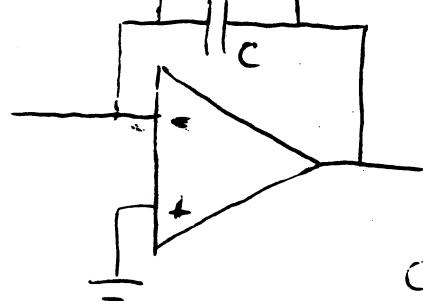
High pass filter necessary to prevent buildup of dc charge on capacitor due to thermal drift and imbalance in op amp
