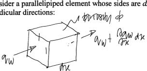
In time dt, the flow of water into the element on the left is  $q_w dt$ , and the flow out of the element on the right is  $(q_w + (\partial q_w / \partial x) dx) dt$ . The volume of the pore space is  $\varphi dx$ , and the volume of water in the pore space is  $\varphi S dx$ . In time dt, the change of the volume of water in the pore space is  $\varphi(\partial S/\partial t)dtdx$ . Since water is essentially incompressible, by conservation of volume
