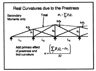
Fictitious equillibrium systems – moments and reactions  $M^*_i = \beta_i Q^*_i$   $N^*_i = \beta_i Q^*_i$  System 2  $N^*_i = \beta_i Q^*_i$  One such system for each internal support
