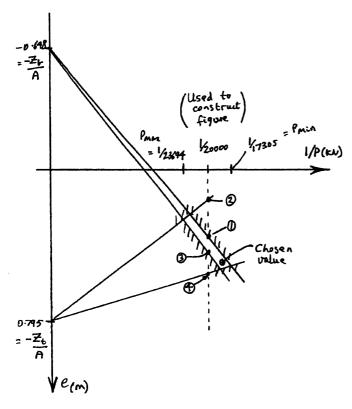
From Magnel diagram find  $P_{min} = 17305$  kN at e = 0.5 m (This value by calculation – accept  $\pm 2\%$  by drawing)
