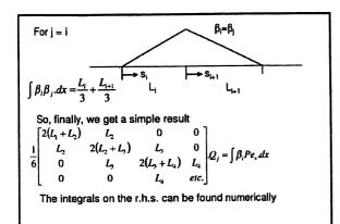
For 2-span beam, only one indeterminacy, so only one equation to solve
