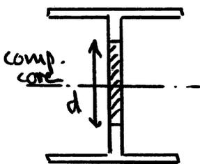
$$P = \sigma_y \times d \times (0.0165) \sim \text{web thickness}$$
