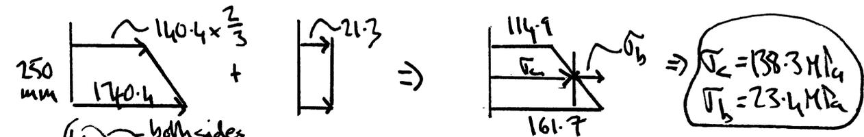
$$\tau = \frac{1}{2} \times \text{both sides} \times 2000 \text{ kN} / [6000 + 21000] \times 10^{-6} = 37.0 \text{ MPa}$$
