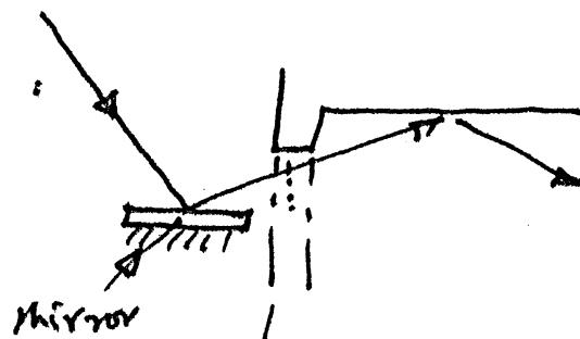
light from more vertical directions (brighter sky) is reflected into top of room through top of window reflects from (hopefully high reflectance) ceiling — then round room to back. Slightly outweighed by obstruction to other light — but that from lower angles less bright. Efficacy — discuss in terms of daylight factor, average for room etc
