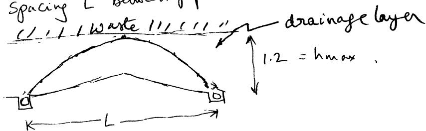
$$L = 2 \times h_{\max} \times \sqrt{\frac{k}{q}} \quad (\text{from data sheet})$$
