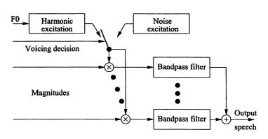
(a)(ii) The channel vocoder is based on the source filter models. The fundamental frequency F0 is detected, together with a decision whether the sound is voiced or unvoiced. The vocal tract response is represented in estimates of the magnitude of the spectrum in a number of filter bands. The filter bands are narrow enough that decimation is used to downsample the output of each filter.
