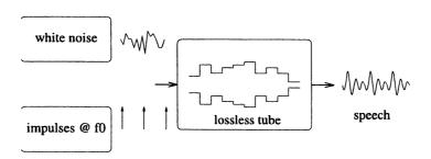
The prediction error sequence can be thought of as excitation to an all-pole model of the vocal tract. The excitation is either quasi-periodic or 'white noise', for voiced or unvoiced speech, respectively.
