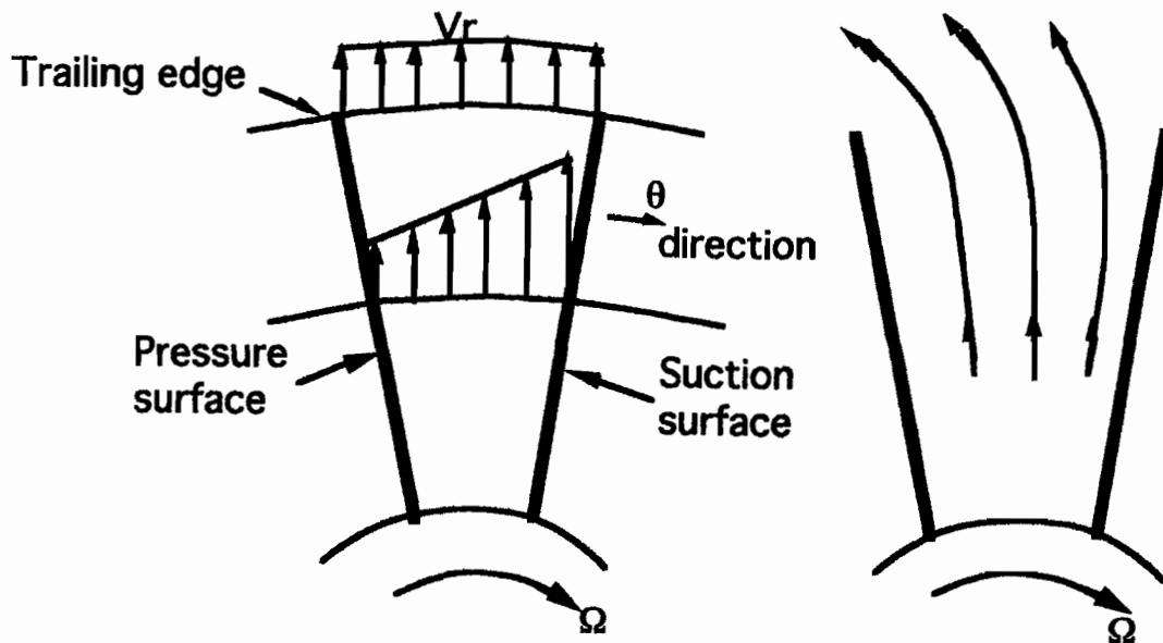
Flow moving radially outward is increasing its angular momentum. There is thus a cross-passage pressure gradient to balance this, with attendant velocity profile. [Sometimes referred to as blade loading]. As the trailing edge is approached, this blade loading drops to zero (a velocity profile becomes uniform) and the angular momentum of the fluid remains constant for further radius change. [20%]
