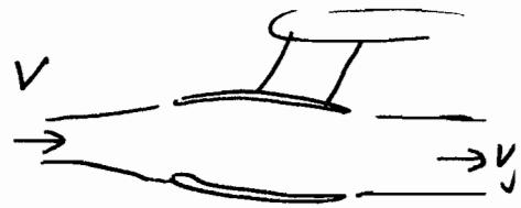
In level flight at constant speed, thrust = drag
