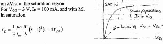
At the onset of saturation,  $V_{DS} = V_{GS} - V_T = 3 - 1 = 2 \text{ V}$ The circuit will operate satisfactorily from this V<sub>DS</sub> up to the onset of avalanche breakdown! At the lower limit of V<sub>DS</sub>,
