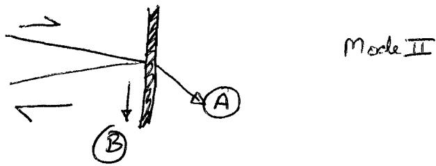
$$\text{The normal stress is } \sigma_{\infty} = -\frac{3}{2} \frac{K_{II}}{\sqrt{2\pi r_2}} \cos \frac{\theta}{2} \sin \theta$$
