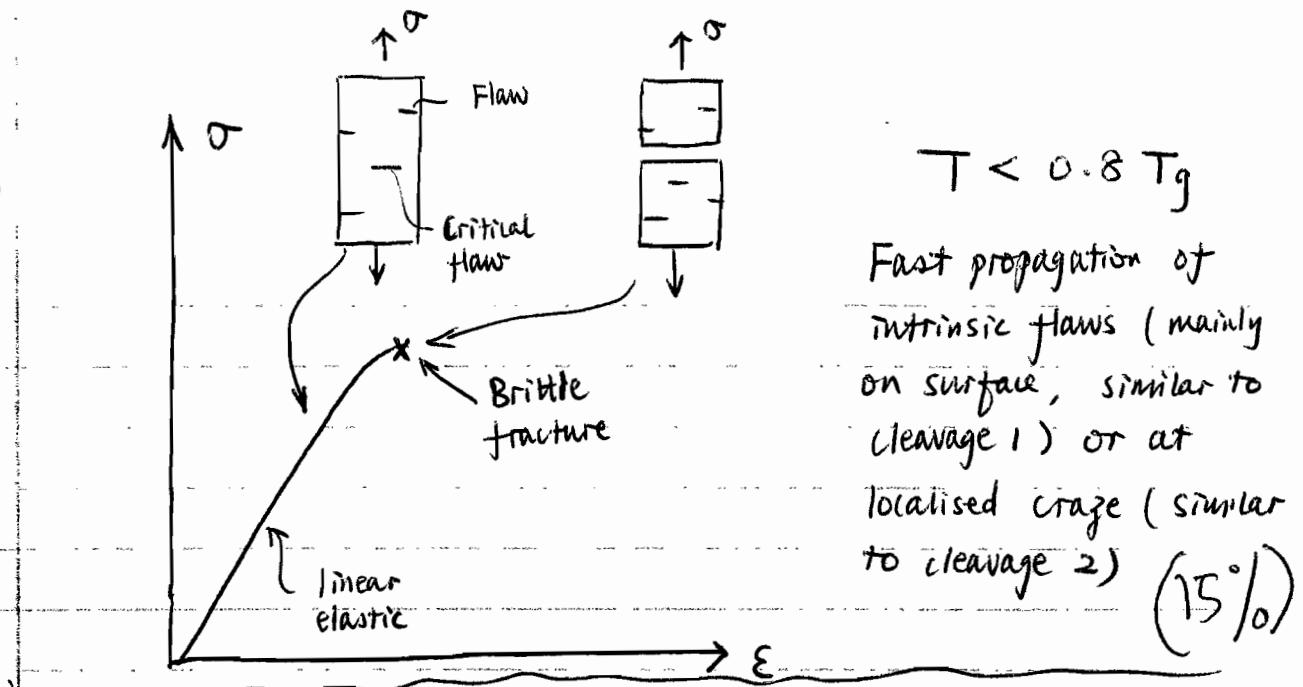
Fast propagation of intrinsic flaws (mainly on surface, similar to cleavage 1) or at localised craze (similar to cleavage 2) (15%)
