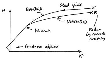
For both beams the behaviour up to first cracking will be very similar. There will normally be some negative curvature when prestressed due to the eccentricity of the tendons. The beams will behave linearly elasticly until the tensile stress capacity is first exceeded.
