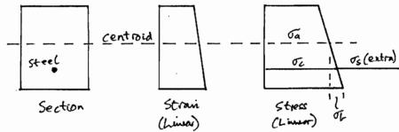
Change in strain in concrete next to tendon = change in strain in steel
