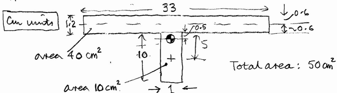
[N.B. If  $\lambda$  for top flange is worked out instead for full width, the T-section is 39 cm wide --- but resulting value of  $\lambda$  (see over) is 53 -- hardly different.]
