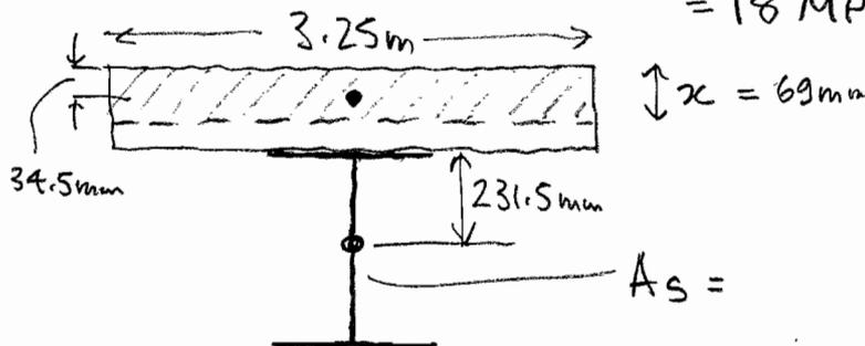
Full plastic tension in steel = full plastic compression in depth  $x$  of concrete.
