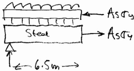
Shear studs together have to carry total force  $A_{sT}$ .
