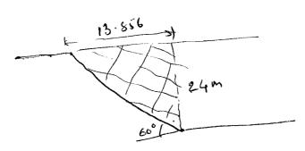
Weight of the waste in the sle  $= \frac{1}{2} \times 24 \times 13.856 \times 100 \times 8 \text{ kN/m}^3$
