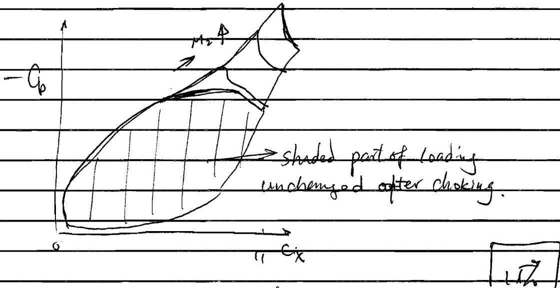
(ii) The limit loading condition is when the passage shock on the suction surface reaches the trailing edge of the blade. Further reduction of the back pressure can no longer have an effect on the surface static pressure distribution. Thus the loading can no longer be further increased. This condition is determined by the exit axial Mach number reaches to unit.
