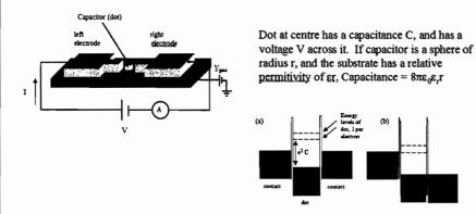
Idea: energy to place electron on island =  $(Q^2/(2C))$ . If this > thermal energy  $(k_BT)$ , can put one electron on at a time, and control this using a gate electrode.
