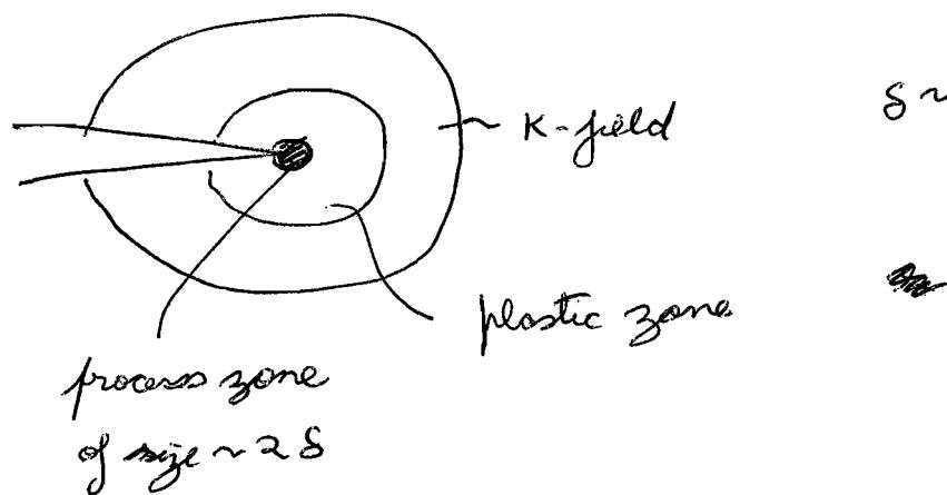
$$\delta \approx \frac{K^2}{\sigma_Y E} = \text{crack opening displacement}$$
