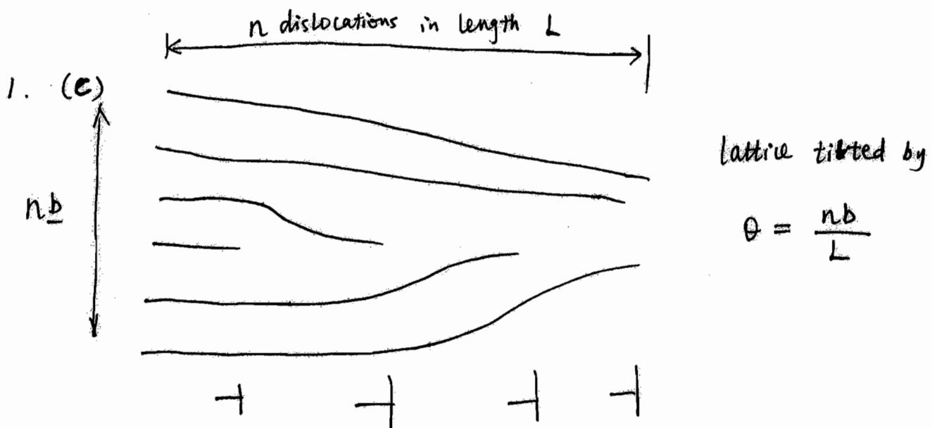
Tilt boundaries separate parts of the crystal which are in slightly different orientations, so they can actually be defined as grain boundaries. The grain size of the material can thus be reduced by cold deformation.
