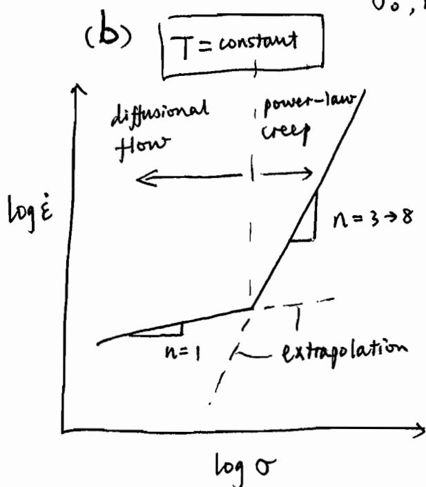
As shown, the extrapolation of power-law creep data may lead to enormous errors in predicting the creep-rate if diffusional flow is overlooked.
