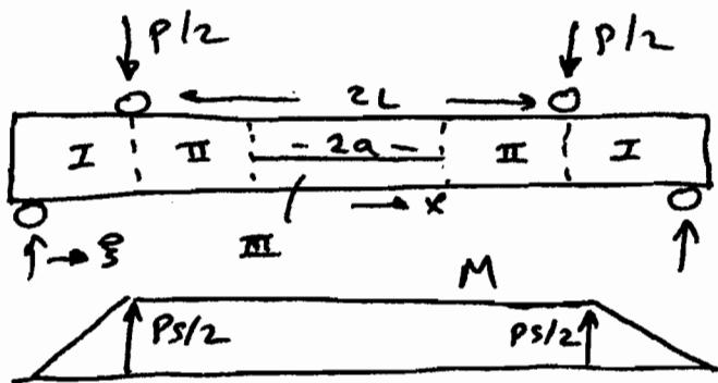
In zone II,  $M = Ps/2$ , thickness =  $t$ , length =  $2(L-a)$
