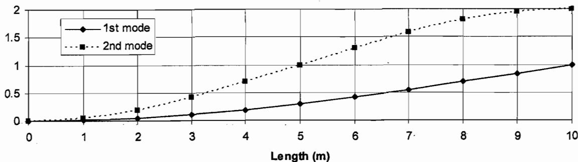
Note: As these are arbitrary mode shapes, the ordinate can be scaled to give unity at the free end of the beam. [20%]
