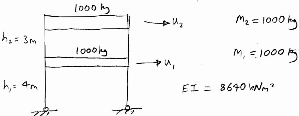
$$K_1 = 2 \times \frac{3EI}{h_1^3} = \frac{2 \times 3 \times 8640}{4^3} = 810 \text{ kN/m}$$
