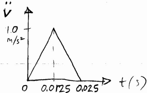
For  $\omega_1$ ,  $\frac{t_d}{T_1} = \frac{0.025}{0.316} = 0.08 \therefore \text{DAF} = 0.2$
