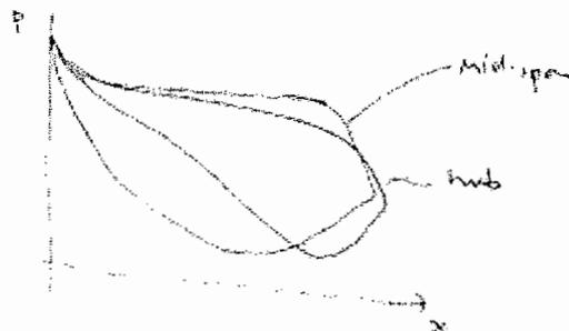
Sweep reduces LE loading at hub and increases TE loading. This is because pressure gradient normal to endwall is small: there is no blade (no loading) away from wall at hub TE, so this is maintained at the wall, reducing LE loading:
