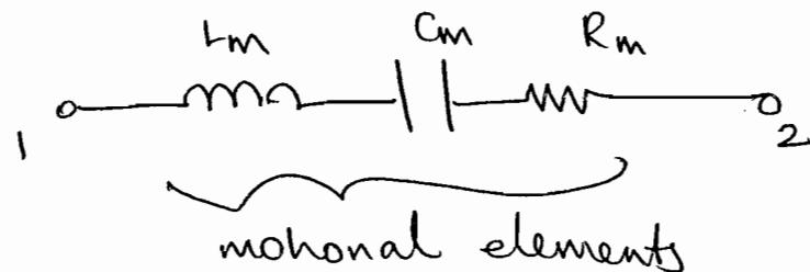
$$L_m = \frac{m_{\text{eff}}}{\eta^2}, C_m = \frac{\eta^2}{k_{\text{eff}}}, R_m = \frac{b}{\eta^2}$$
