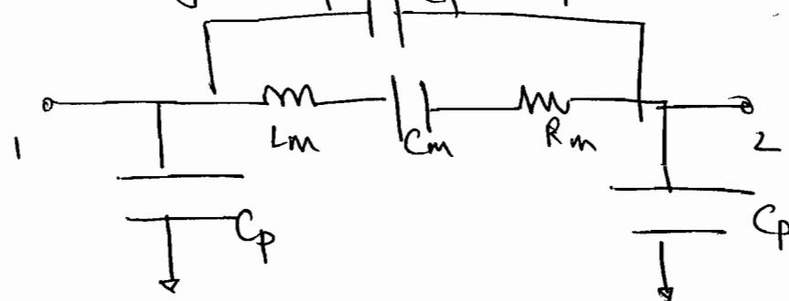
$C_p$  - parasitic capacitor that couples electrical signal to ground.
