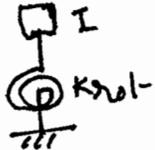
Mass moment of inertia  $I = 180000 \text{ kg-m}^2$
