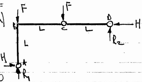
$$\begin{aligned} \Rightarrow R_1 + R_2 - 2F &= 0 \\ R_1 + 2R_2 - F &= -H \\ R_1 - F &= H \end{aligned} \quad \left. \begin{aligned} R_2 &= 0 \Rightarrow R_1 = 2F, H = F \end{aligned} \right\}$$
