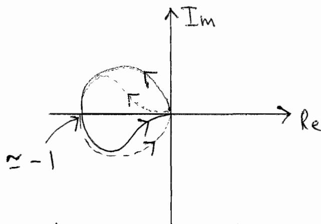
At  $\omega$  slightly greater than 1 rad/sec  $\not\propto G(i\omega) = -180^\circ$  and  $|G(i\omega)|$  is (slightly less than) 0 dB.
