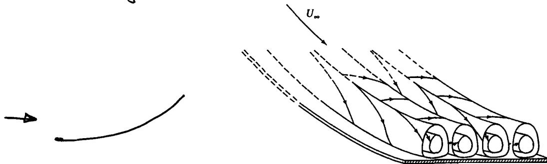
On the convex side, the mean flow is slowed down and so there is an adverse pressure gradient. This will result in a somewhat thicker boundary layer.
