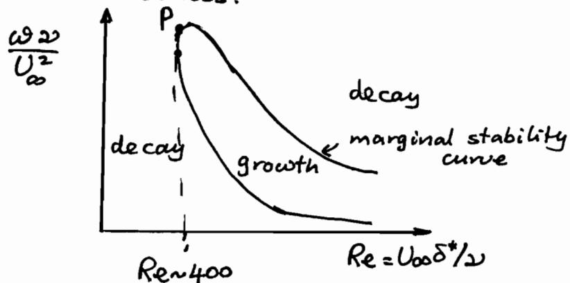
Near the leading edge, disturbances of any frequency decay. At a particular distance  $x$ , downstream of the leading edge corresponding to  $\delta^*(x) \approx 400/U_\infty$  one frequency becomes unstable (position P on the curve). However a disturbance of this frequency travels downstream where the boundary layer is thicker and the disturbance decays. Further downstream a range of frequencies will be amplified and Tollmien-
