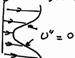
Other examples are mixing and jet flows and convection near a hot stationary wall.
