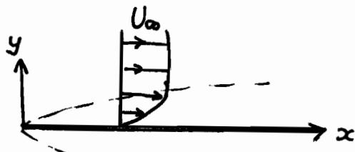
The Blasius profile for a laminar boundary layer is self-similar and the mean velocity profile can be written
