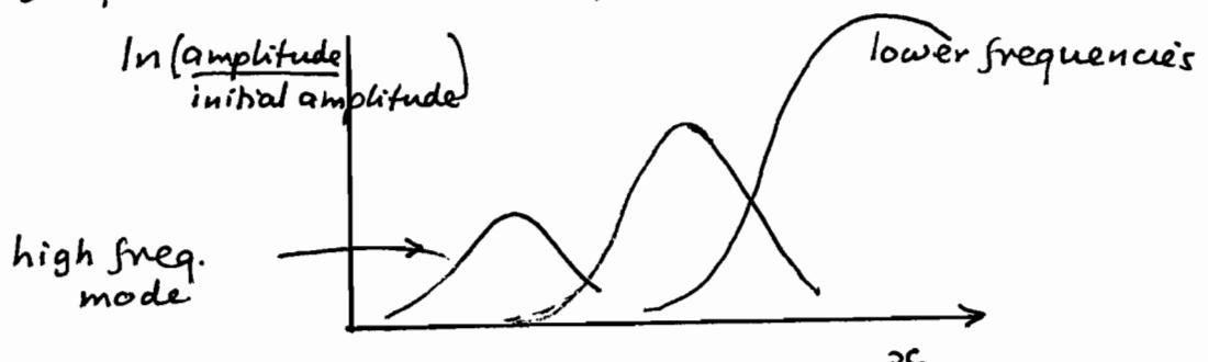
Schlichting waves will be seen. Once the wave amplitude exceeds a critical value, nonlinear and three-dimensional effects become important. Complex flow structures appear which ultimately lead to turbulence.
