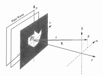
If we consider an infinitely small differential of the aperture, dS, we can model this as a point source of light emitting spherical 'Huygens' wavelets with an amplitude of A(x,y)dS. The wavelet acts as a radiating point source, so we can calculate its field at the point P, a distance r from dS. The point source dS can be considered to radiate a spherical wave front of frequency  $\omega$ .
