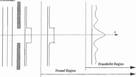
b) We want to calculate the far field or Fraunhofer region for a square aperture. This aperture can be represented in two dimensions as a 'block' function.
