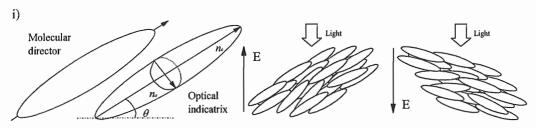
ii) Based on the geometry of the optical indicatrix, the light (polarised parallel to  $n_{\rm e}$ ) passing from above sees an average of the two components of the refractive index.
