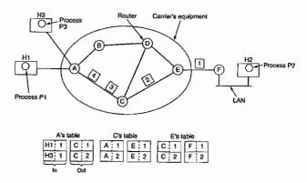
to that used in source routing systems. Hence a MPLS router will receive a frame, read its label and look it up in a simplified table to determine the next hop in the route. The VC label is not always constant across the route as it may have to be updated in order to manage similar MPLS packets using the same routes from different flows.
