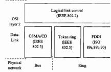
The LLC provides direct (OSI layer 2) connection between any two end devices locally connected to the LAN. It made sense to define a standard interface
