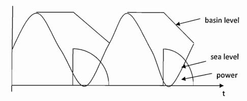
Graph shows how these schemes produce bursts of large amounts of power but for relatively short periods, say 6 hours. By increasing the diversity of supply eg by connecting in a similar scheme which has high tides at opposite times this effect is reduced. By strengthening the grid at the location of the scheme the power can be exported to where it is needed.
