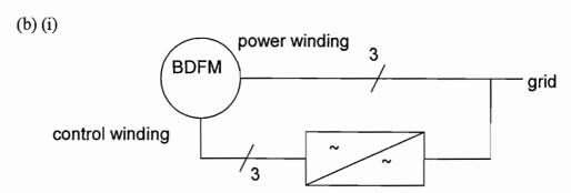
Key features in diagram are direct connection of power winding to the grid, and the connection of the control winding via a bi-directional converter giving a variable voltage, variable frequency feed.
