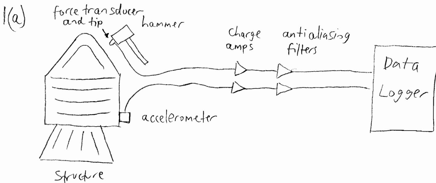
(i) Hammer mass  $m$ , tip stiffness  $k$  produces a half-sine force pulse of duration  $b = \pi\sqrt{\frac{m}{k}}$
