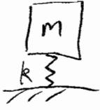
the piezo force element has a stiffness  $k$  so the accelerometer has a resonance at  $\sqrt{\frac{k}{m}}$
