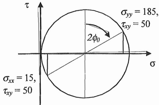
So, at the origin the stress is equivalently described by  $P_o = 100\text{MPa}$ ,  $k = 100\text{MPa}$ ,  $\phi_0 = \pi/6$ .  $k$  is a material constant.
