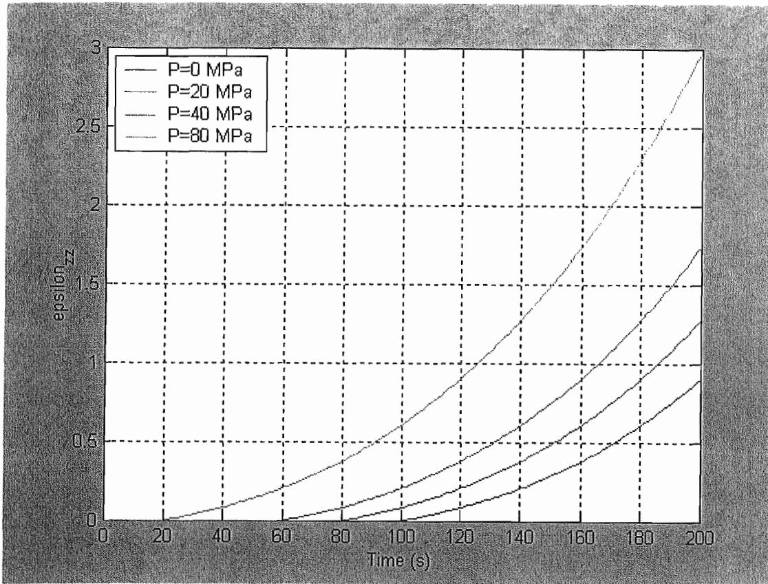
Increasing pressure leads to earlier yield, and greater extension for a given stress along the wire.
