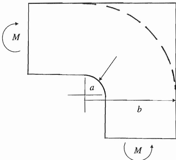
Material outside dashed line cannot add significantly to mechanical strength of component - so assume two stress free
