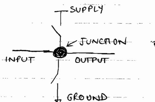
In this case, the relative resistance from INPUT TO JUNCTION, OUTPUT TO JUNCTION & FROM these points to supply and ground define switching together with the magnitude of  $V_{PI}$ .  $V_{PI}$  needs to be small for low voltage switching and devices can switch quickly if their dimensions are reduced.
