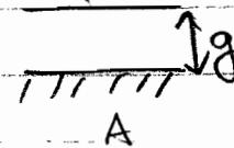
$$F_{\text{mech}} = k(g_0 - g) \quad F_{\text{elec}} = -\frac{\partial W}{\partial g} = \frac{\epsilon_0 A V^2}{2g^2}$$
