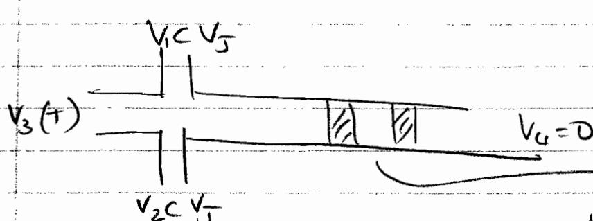
Next switch the field off between ports 1 and 2 and drive a plug of sample from 3 to 4
