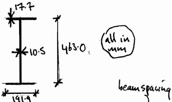
Floor spans 14 m, simply supported  $\Rightarrow$  effective width =  $\frac{14}{4}$  or 3.5 m
