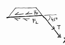
Force on uppersurface of geomembrane Fu = Tran Su = 14 x1x Tan 5°x1 = 1.225 KN.
