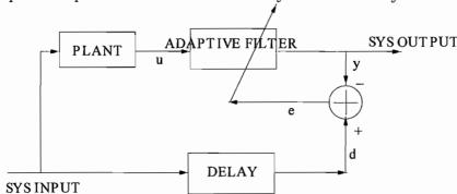
*Prediction:* The function of the adaptive filter is to provide the best prediction (in some sense) of the present value of the input signal. The input of the filter are the past values, hence the delay. The desired response is the present value.
