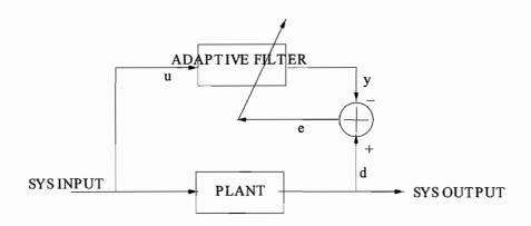
Inverse modeling: The function of the adaptive filter here is to provide the best fitting (in some sense) inverse model to the unknown noisy plant. Ideally the inverse model will have a transfer function equal to the inverse of the plant's transfer function. The desired response is a delayed version of the plant's input. In some instances a delay is not necessary.
