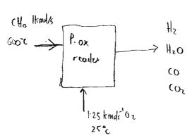
Need markerial bulance to calculate mular Hows out of reactor.
