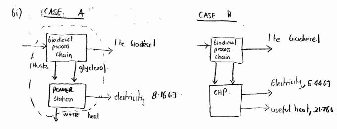
total energy input to ponerstation or eff is  $1.5 \times 17 + 0.1 \times 17 = 27.265$  CASEA 5 electricity output =  $0.3 \times 27.2 = 8.1865$
