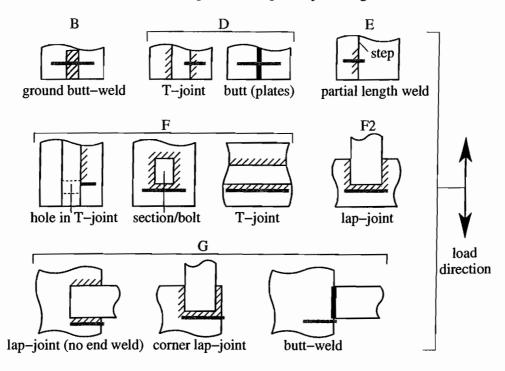
e. Weld fatigue life. The number of repetitions, N, to failure under stress amplitude,  $\sigma_r$ , is
