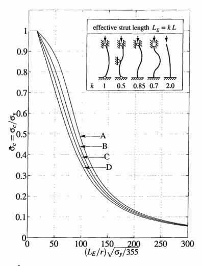
**note 1:**  $\sigma_y$  in N/mm<sup>2</sup>; r is the radius of gyration about centroid of cross-section; curves are selected as follows (linear interpolation used for intermediate r/y values.)
