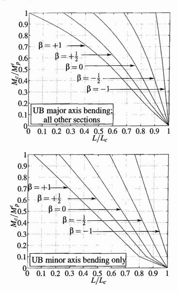
**note 1:**  $M_p'$  is the reduced plastic moment;  $\beta$  as in DS2;  $L_c$  is the length of a pin-ended column buckling under P alone (found with DS1); only use CDC method if  $\lambda_{\text{web}} \leq 56$ .
