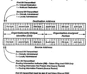
(c) The MAC address has a standardised 48 bit structure which has been adopted as part of the IEEE 802 set of LAN protocols. The address can identify both the transmitting station (source address) and the receiving station (destination address).
