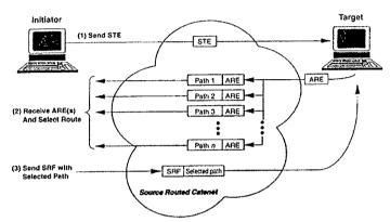
AREspecifically request, routed response - The sending station send an ARE frame which will arrive af the destination by multiple recorded routes. The receiving station selects a route and sends a SRF back to the sender to indicate the chosen route. This places a processing burden on the receiver, so a variation of this is for the receiver to send
