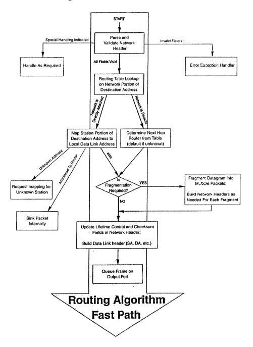
Routing table look up – The router performs a table look up to determine the output port to direct the packet to, based on the network identifier of the IP address. The result of this will be that either:
