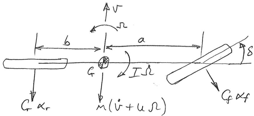
$$(a) \sum F: m(v + uR) + C_f \alpha_f + C_r \alpha_r = 0 \quad \left. \begin{array}{l} \\ \end{array} \right\} \quad (1)$$
