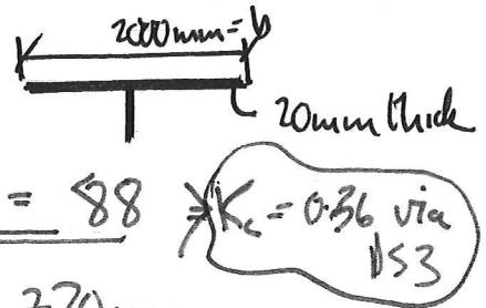
$$\text{Effective section has } b_e = K_c \cdot b \text{ or width } h_e = 720 \text{ mm}$$
