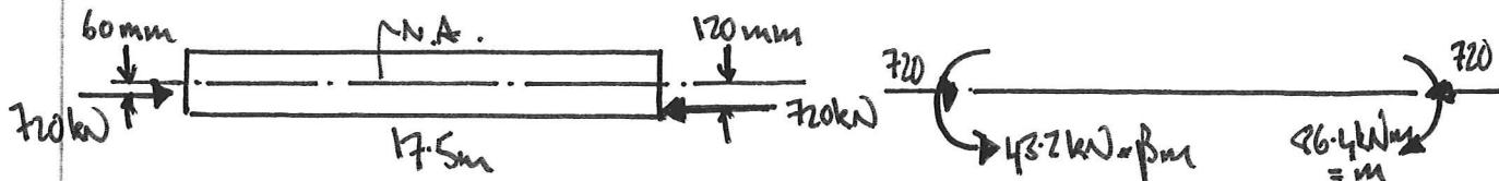
$$\text{Ratio of end moments} \Rightarrow B = 1/2 : \Rightarrow M_B = (0.6 + 0.4 \times 1/2) m = 0.8m$$
