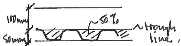
Effective width of span = smaller of  $\frac{1}{4}$  span or  $\frac{3}{4}$  beam spacing : 3m
