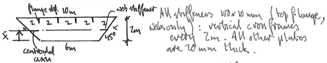
$$\text{Smeared thickness of top flange: } 10 \times 0.02 + 4 \times 0.1 \times 0.01 = 10h \Rightarrow h = 20.4 \text{ mm}$$
