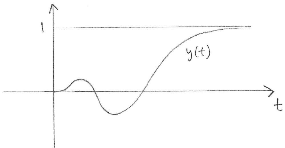
Initial slope zero, but moving up due to positive 2<sup>nd</sup> derivative. RHP zero(s) implies output must go to zero at some time.
