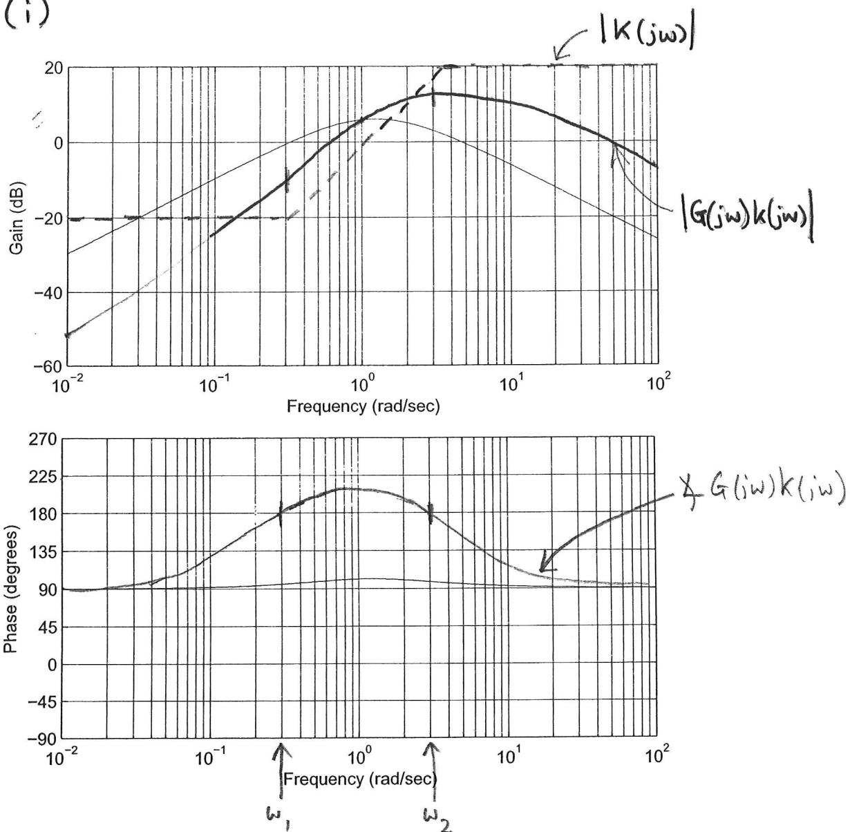
(ii) Notice that  $|k(i\omega)| < 1$  for  $\omega < 1$  and  $|k(i\omega)| > 1$  for  $\omega > 1$ . There are two frequencies  $\omega_1 < \omega_2$  where  $\angle(G(i\omega)k(i\omega)) = 180^\circ$ . So  $|G(i\omega_1)k(i\omega_1)| < 1$  and  $|G(i\omega_2)k(i\omega_2)| > 1$ .
