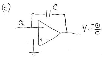
The gain of the charge omplifier is - = where C is the feedboot caponitone
