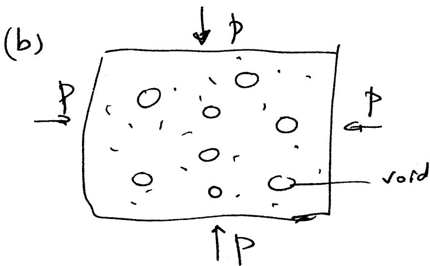
plastic deformation can occur between voids and give rise to a macroscopic change in volume due to the change in void size.
