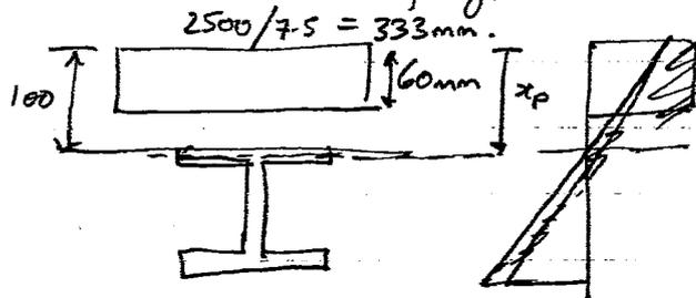
$$x_p \left( \underset{\text{conc}}{333 \times 60} + \underset{\text{steel}}{7650} \right) = \left[ \underset{\text{conc}}{333 \times 60 \times 30} + \underset{\text{steel}}{7650 \times \left( \frac{100 + 406.4}{2} \right)} \right]$$
