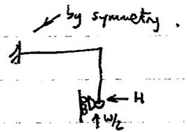
Pick H as redundancy: Statically Determinate system.
