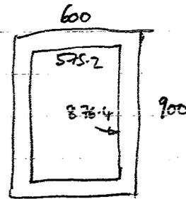
$$I_{\text{major}} = \left( \frac{bd^3}{12} \right)_{\text{ext}} - \left( \frac{bd^3}{12} \right)_{\text{int}} = \frac{1}{12} \left[ 600(900)^3 - 575.2(876.4)^3 \right] = 4184 \times 10^6 \text{ mm}^4$$
