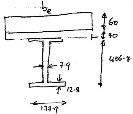
SDB:  $A_{steel} = 76.5 \text{ cm}^2$  ;  $\text{mass/m} = 60.1 \text{ kg/m}$   $I_{major} = 21600 \text{ cm}^4$
