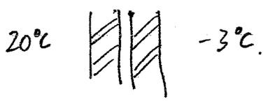
$$q = U \Delta T \rightarrow q = (0.34 \text{ W/m}^2\text{K})(23 \text{ K}) = 7.82 \text{ W/m}^2$$
