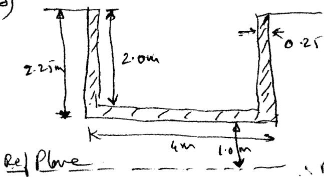
$$\text{Volume of concrete in side walls} = (4^2 - 3.5^2) \times 2 = 7.5 \text{ m}^3$$
